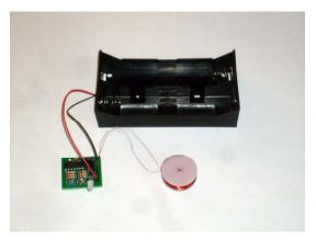
The pendulum drive electronics consists of a battery box, circuit board with microcontroller, and coil.
