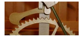
For this mechanism to function properly, the back-and-forth movement of the driving pawl must be within a certain range of travel. Too little, and the pawl won't pull the ratchet wheel far enough for it to jump to the next tooth on the wheel. Too much, and the pawl will jump two or more teeth.
